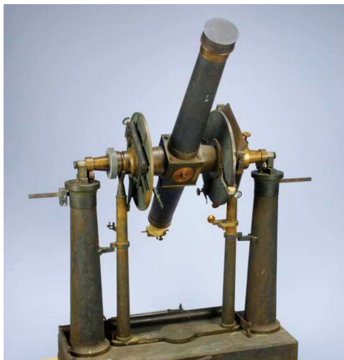
Figure 8 — Fauth & Co, surveyor telescope ca. 1880. (public domain)
